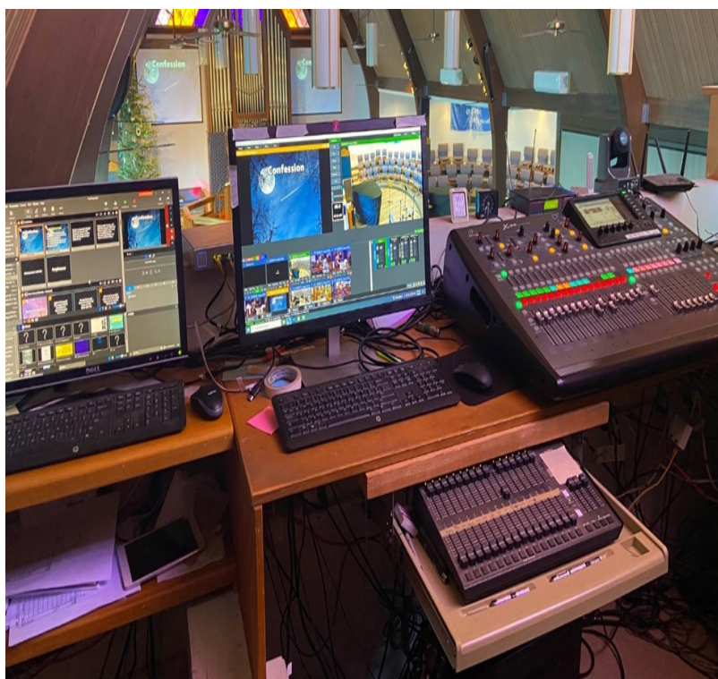
Equipment up in sound booth. From left PC for projection (ProPresenter), PC for video editing (vMix) and also Zoom broadcast, Mixer board for sound Behringer X32, and below control panel for spot lights.
